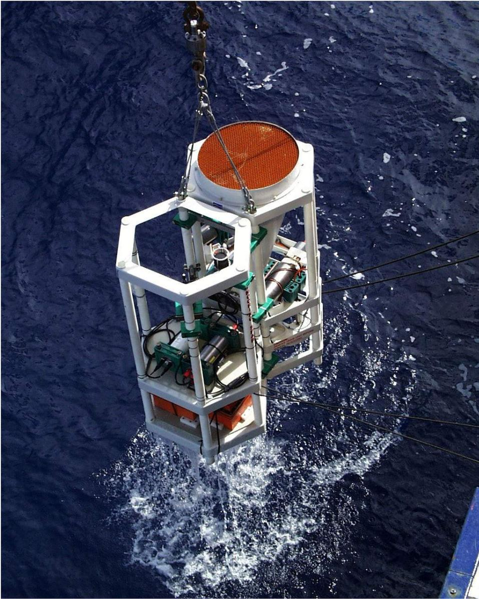
Fig 4: Multi Sensor Device MSD during tests at ships wire.
