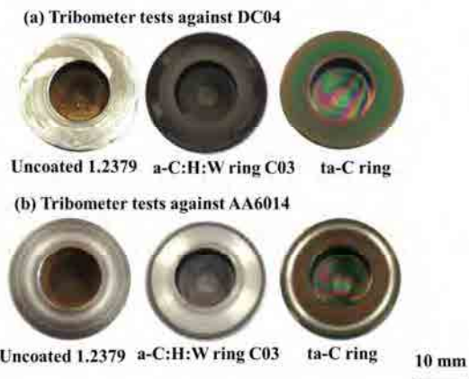
Fig. 12: The wear tracks on tested rings against (a) DC04 and (b) AA6014
