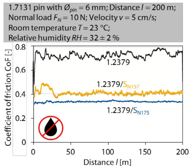
Figure 7: Coefficient of friction of the uncoated 1.2379 substrate and coated samples 1.2379/S<sub>N157</sub> and 1.2379/S<sub>N175</sub> against 1.7131 using PoD tribometer
