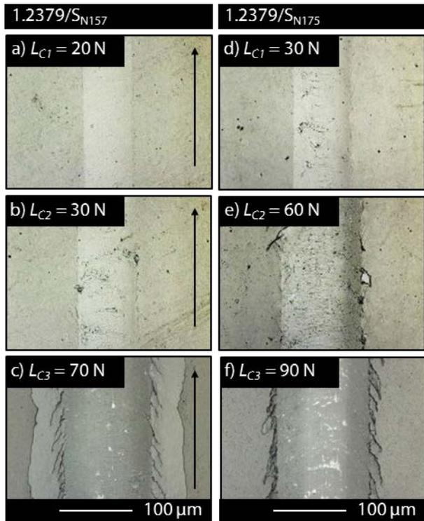
Figure 6: CLSM micrographs of scratch tracks on 1.2379/S<sub>N157</sub> (a-c) and 1.2379/S<sub>N175</sub> (d-f) after scratch tests with critical loads  $L_{C1}$ ,  $L_{C2}$  and  $L_{C3}$
