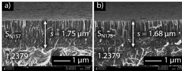
Figure 3: SEM cross section fractures of the  $\text{S}_{\text{N}157}$  (a) and  $\text{S}_{\text{N}175}$  (b) coated 1.2379 substrates
