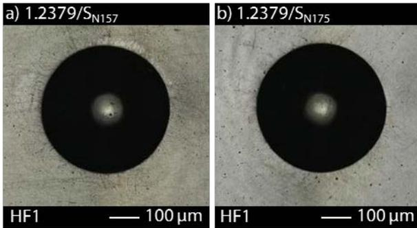
Figure 6: CLSM micrographs of Rockwell indents on 1.2379/S<sub>N157</sub> (a) and 1.2379/S<sub>N175</sub> (b) for determination of adhesion classes (HF)
