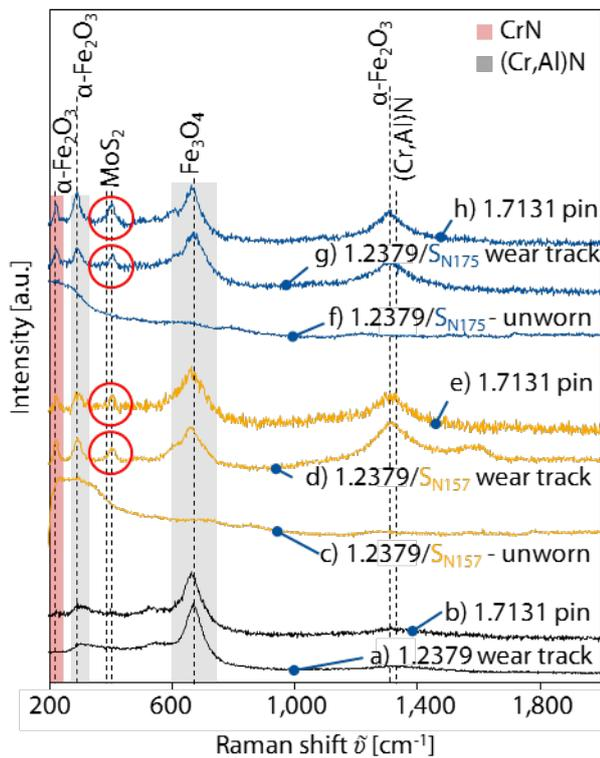
Figure 8: Raman spectra of the uncoated 1.2379 substrate, S<sub>N157</sub> and S<sub>N175</sub> coated samples and counterparts after PoD model tests as well as spectra of as deposited samples
