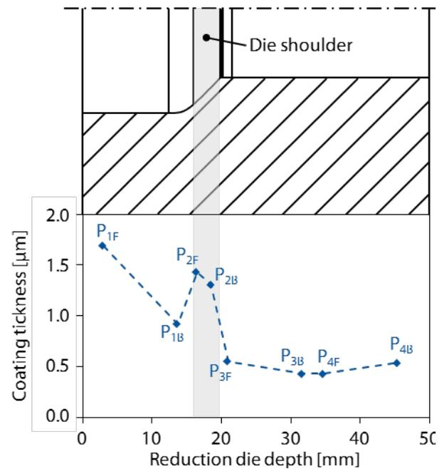
Figure 5: Thickness distribution of the coating S<sub>N175</sub> along the longitudinal axis of the experimental tool
