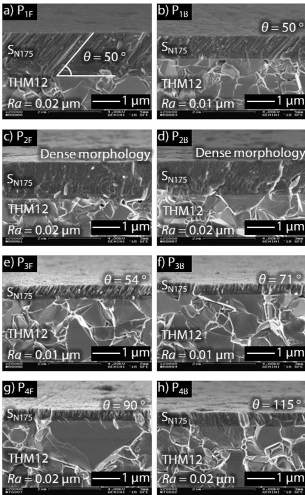
Figure 4: SEM cross section images of the S<sub>N175</sub> coated THM12 substrates positioned at P<sub>1F</sub> to P<sub>4B</sub> (a-h) along the longitudinal axis of the experimental tool and the corresponding values of Ra
