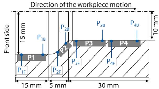
Figure 1: Schematic of the experimental tool and the THM12 substrates at positions 1 to 4
