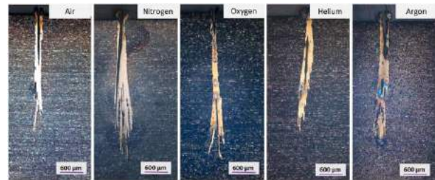
Figure 5: Influence of the process gas on the shape of the borehole at 10 mbar process pressure. Illustrated by micrographs cross sections, etched with Adler.
