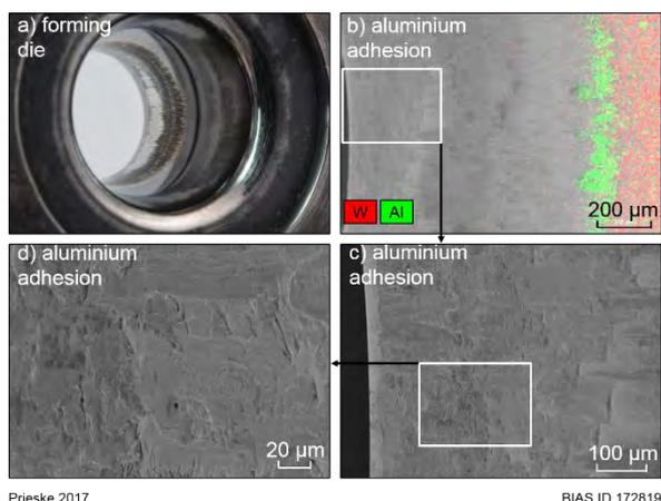
Figure 5: Wear of the forming die after dry tapering a) shows a photo of the forming die, b) an EDX measurement and c) and d) close up images of the adhesion.
